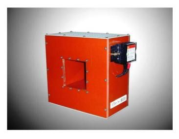
•This demagnetizer can put bench, and use it. Input commercial AC power source into coil directly, and generate alternating current magnetic field. Demagnetize in a range attenuation mode to pass an object in alternating current magnetic field.
