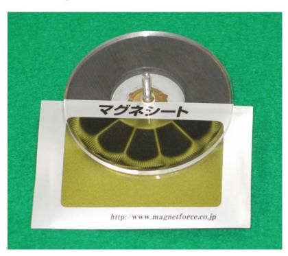
The left pictorial image shows pattern of magnetic pole when multipole magnetized in the circumference region after having done 16 pole magnetizing in a face of a ring type magnet.
